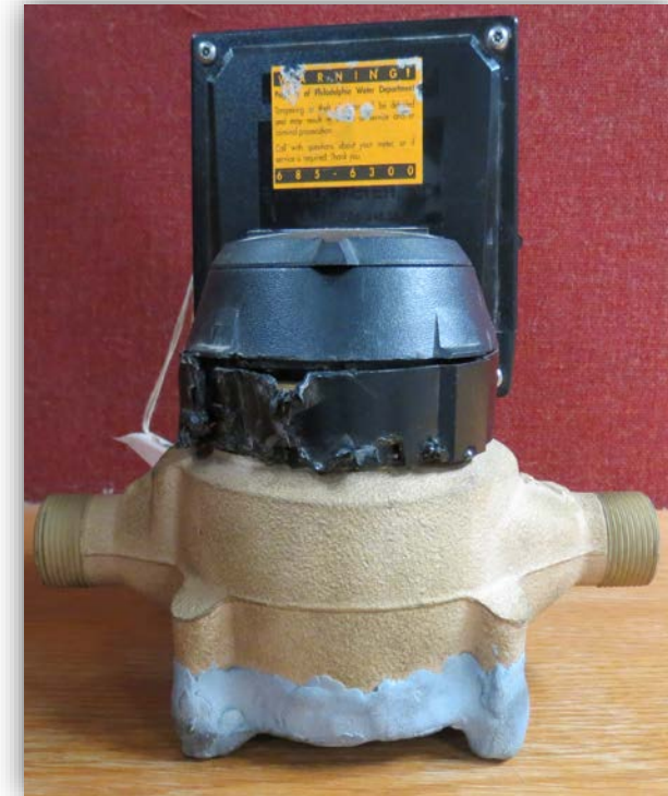
Damaged meter register from attempt to tamper with the meter
