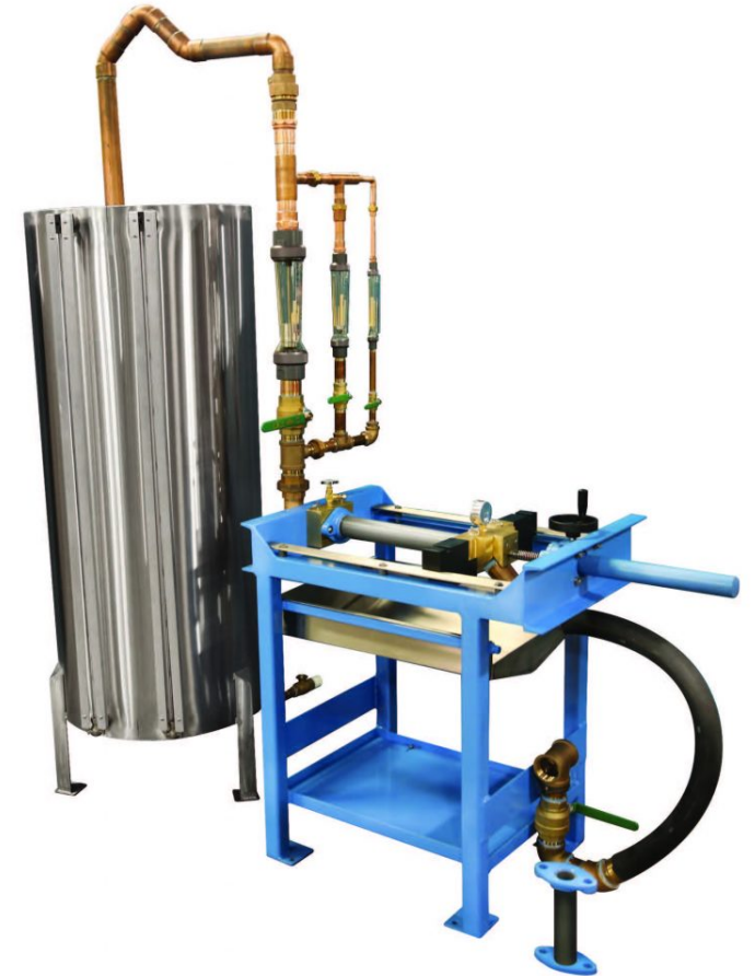
Meter test bench used for testing residential meters of 5/8-inch size Source: Waterfm.com
