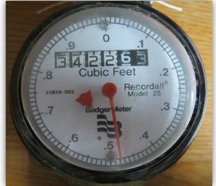
Direct read “odometer” style meter register with sweep hand
