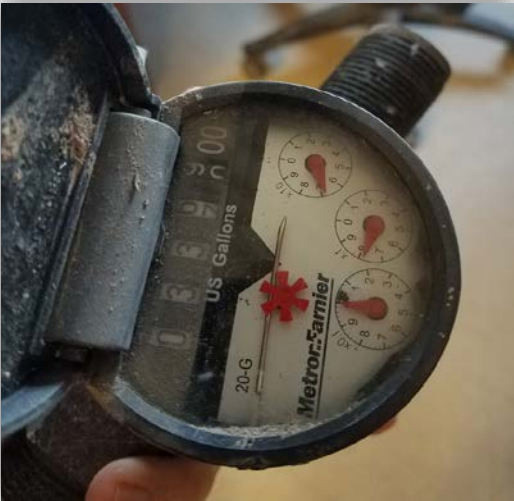
Tampered customer meter with nail inserted into register to slow meter function
