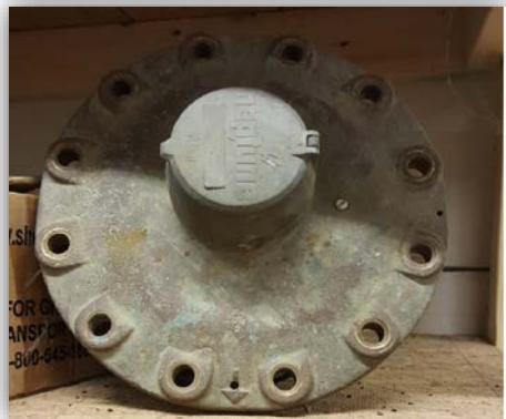
Inter-changeable Unitized Measuring Element (UME) for a large turbine meter
